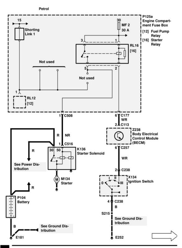
As you can see from the diagram the starter relay is activated by a 0v ground signal from the key via the BECM (Body Electrical Control Module), which interrupts this signal if there is an immobiliser active.
